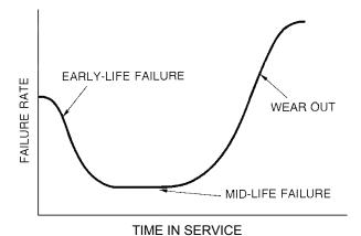
Figure 1.2 The failure rate with time of a group of similar components.
